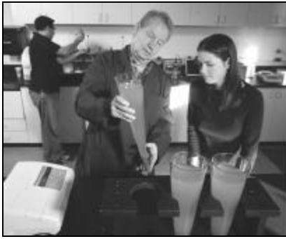
Professor Joe Reichenberger explaining settleable solids - an important characteristic of wastewater.
